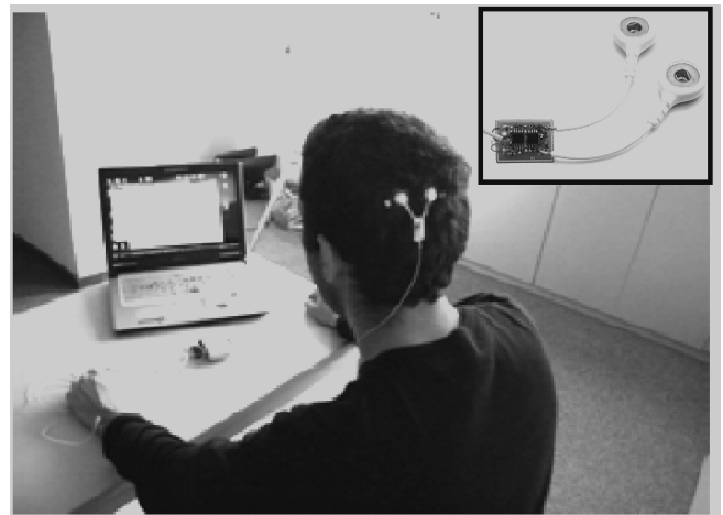
Fig. 2 - Electrodes scheme and acquisition system
